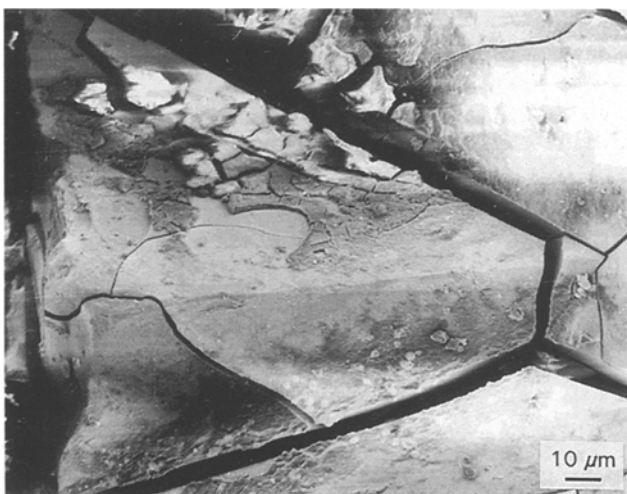
Figure 10 Scanning electron micrographs demonstrating the propagation of vacuum- and electron beam heating-induced cracks bearing no definite crystallographic directions.
